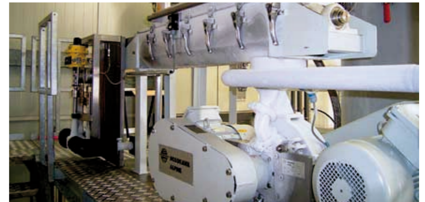
CW CRYOGENIC GRINDING SYSTEM IN CIRCUIT-GAS MODE WITH LN 2
